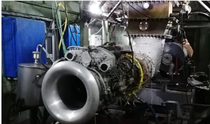
**Fig. 5 TA2 engine on test rig**
