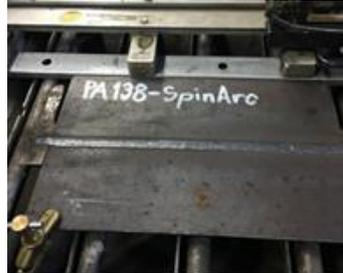
Fig. 12. Welding obtained by the mechanized SpinArc process
