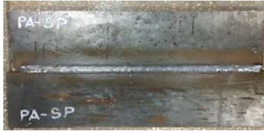
**Fig. 6. Full-shape PA welding**
