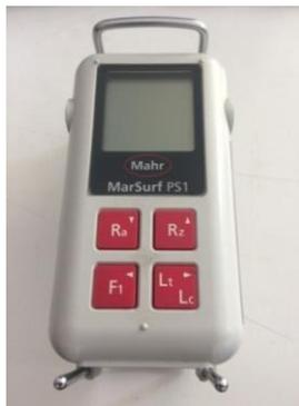
**Fig.3 MarfSurf PS1 roughness tester**
