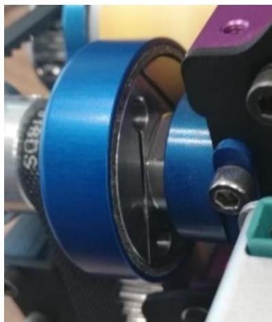
**Fig. 3a Centrifugal Clutch mechanism**
