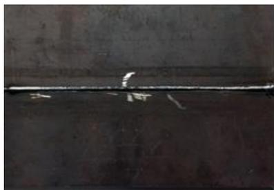
**Fig.10. Root obtained through the SpinArc process**
