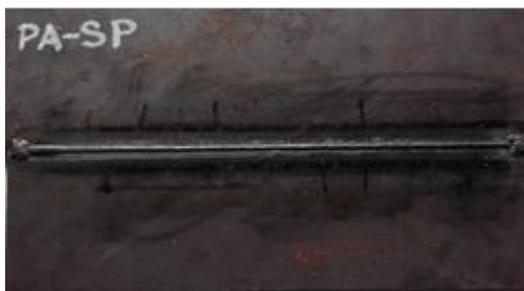
**Fig. 4. PA welding root layer with solid wire**
