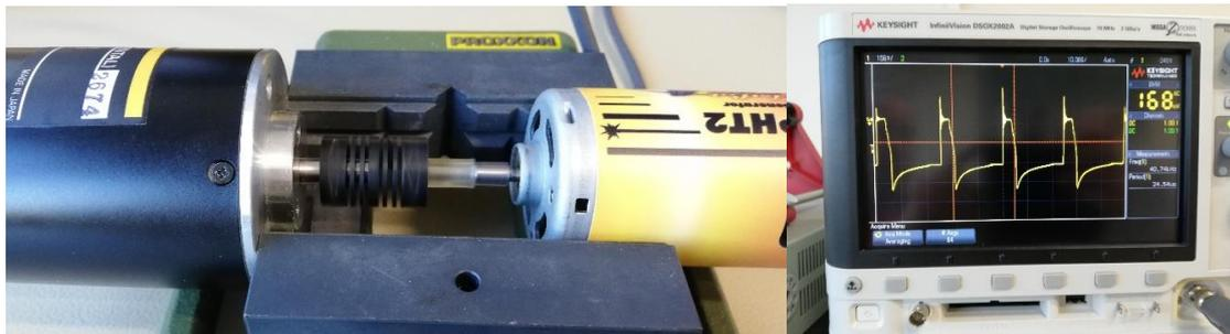
**Fig. 6 Starter Generator testing.**
