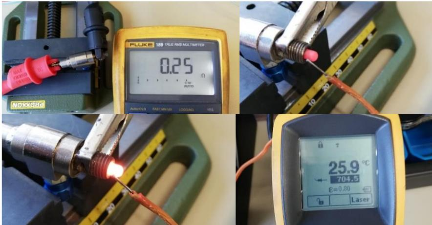
Fig. 18 GP testing (from left up to right down corner: internal resistance, low power glow, maximum power glow, temperature reading of GP tip)
