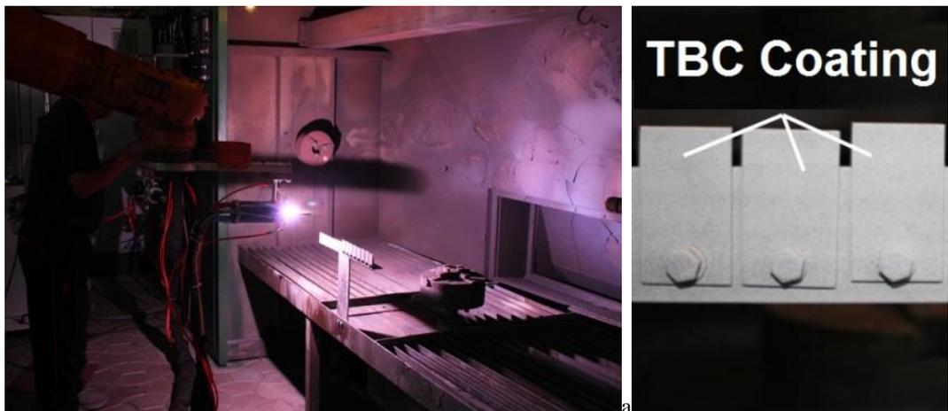
Fig. 2. Thermal spray deposition process of TBCs using Metco 7M installation with F4 gun (a) and the coated specimens (b)
