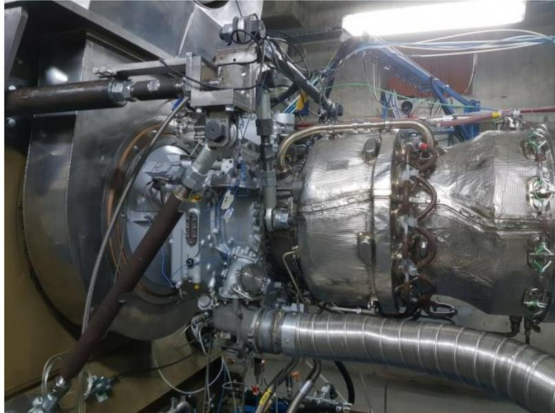
**Fig. 5 Installation of the ST40M engine in the test bench**
