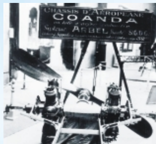
The two Gnome rotary engines of the Coanda Twin, the first multi-engine Airplane, Reims, 1911.
